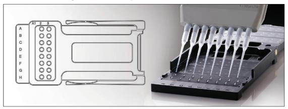
Turn your Cytation 5 into a micro-volume analysis system with Take 3. You can run 16 or 48 samples in one run to save a lot of time compared to single-sample devices. Gen 5 is pre-programmed for ssDNA, dsDNA, RNA and protein quantification in 2  $\mu$ L.
